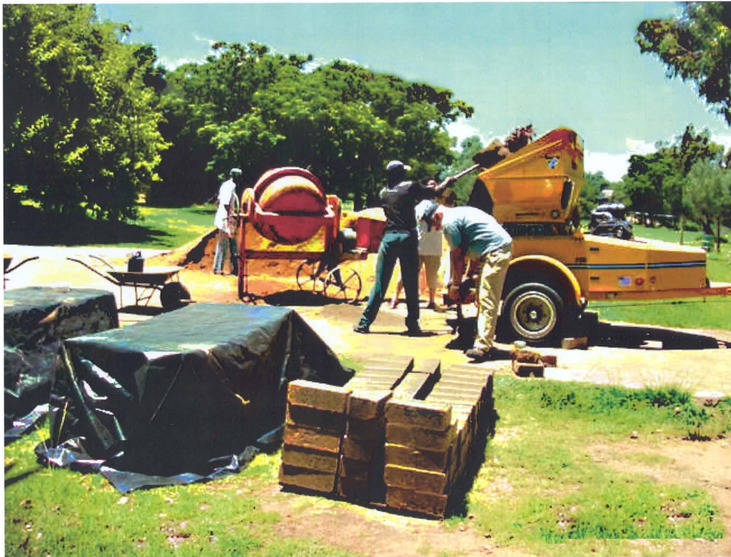
Figure 14: A Compressed Earth Block Machine Intended to Help Build Schools in Kabul, Afghanistan
